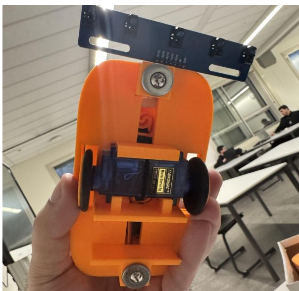
Figure 2: Bottom view showing servo motors and line sensor array
